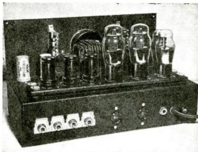
The amplifier rear view, above, shows the tubes mounted on an anti-microphonic base. Unit includes the following features: Variable high and low inverse frequency compensation with concentric constant-current inverse feedback inverter; humless push-pull beam power output; dialogue filter; low-level, noiseless, non-frequency discriminating gain controls (adapted for remote control).
