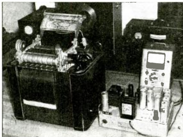
← Recorder mechanism, with printing bar lifted to show inserted stencil and backing paper. At right is the receiver chassis removed from the cabinet. (Test units constitute the background.)
